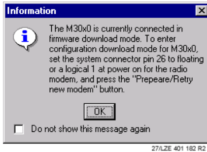
Figure 4 M30x0 radio modem connected in firmware download mode
