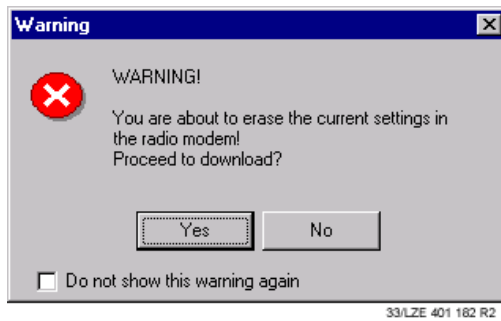
Figure 16 Warning dialog before erasing data from the radio modem.
