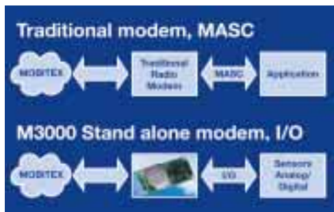
▲ The OAI firmware in the M3000 stand alone modem, I/O, encapsulates the MASC protocol for maximum efficiency. A Java application can use the I/O, D/A, A/D and I 2 C channels for monitoring and control of for example alarms, vending machines and other equipment.
