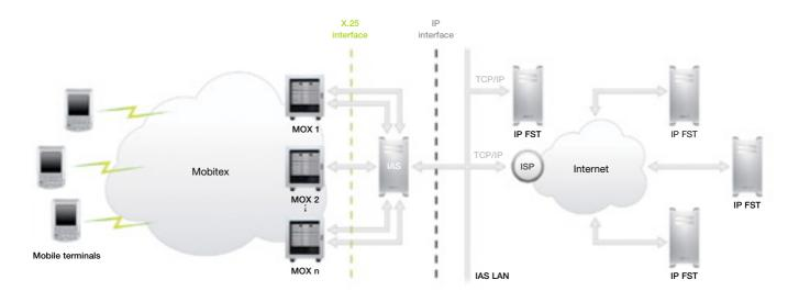
The IAS is connected to a local area exchange (MOX) in the Mobitex network, where it provides an interface between the Mobitex network and IP-connected fixed terminals.
